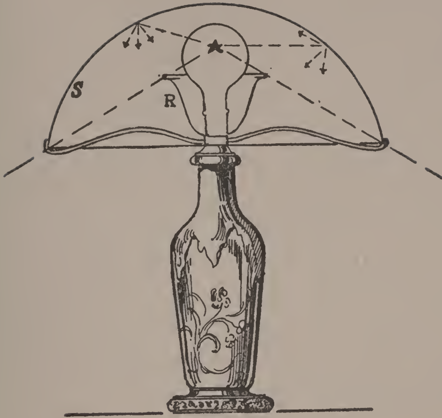
Fig. 13. The light-source is shielded by an opaque reflector, R. The light is reflected from the inner surface of shade, S. Thus, coming from a large area instead of a small brilliant filament, the lighting is less harsh.
